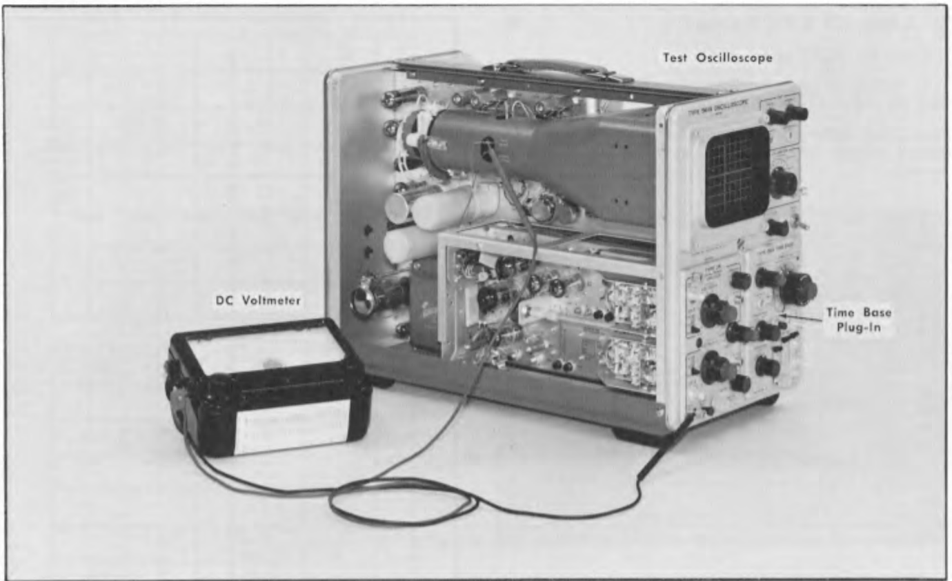
Fig. 7-5. Test equipment setup for step 5.
